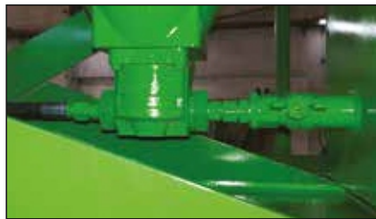
Hydraulic oil pump located outside of the tank for ease of diagnose
